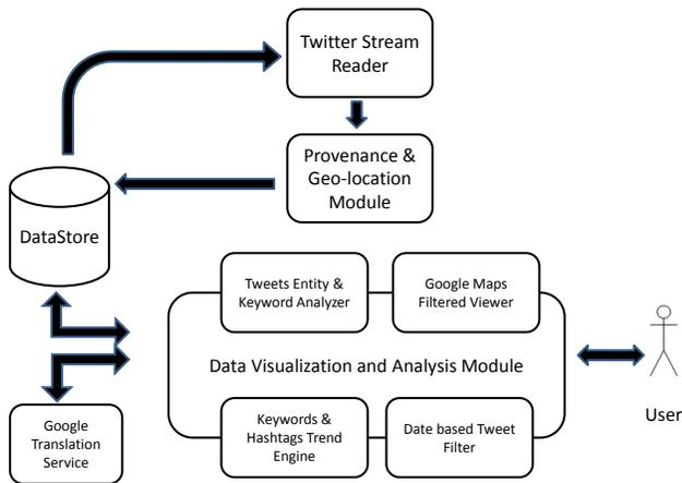
Figure 1: System architecture of TweetTracker
